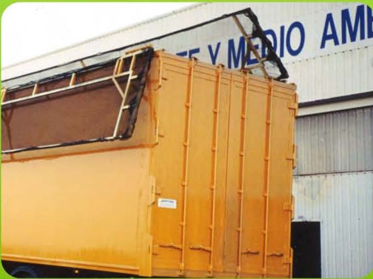
Hydraulic roof opening / Backdoors like a book Aluminium bodywork
