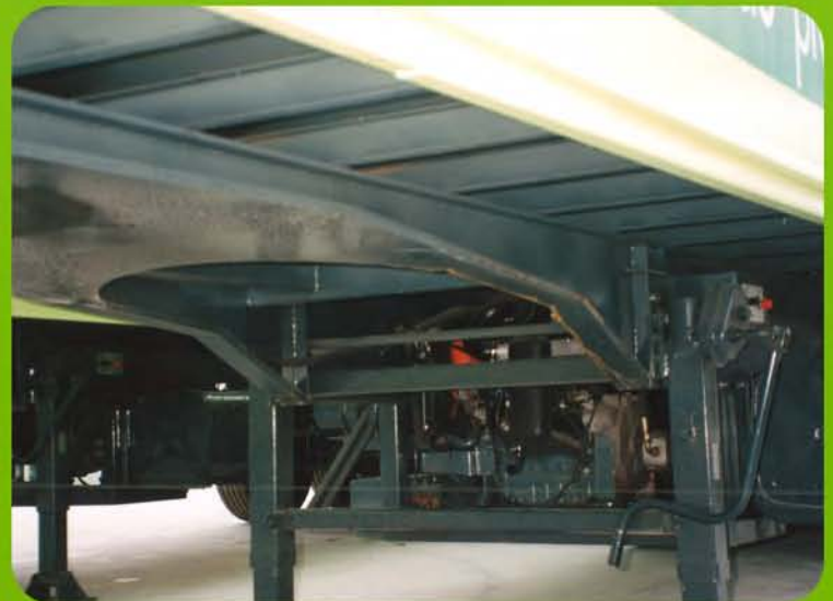
Automatic motor mounted on trailer
